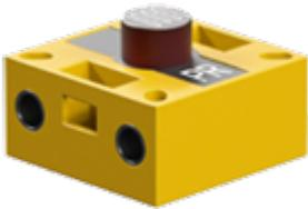
the resistance of the photoresistor drops when it is exposed to more brightness. The value output by the photoresistor, therefore, is a measurement of brightness.
