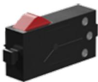
The button is a digital sensor that differentiates “current flowing” from “no current flowing.” Whether current is flowing, therefore, depends both on the wiring and on whether the button is pushed. You can use the button in two ways:
