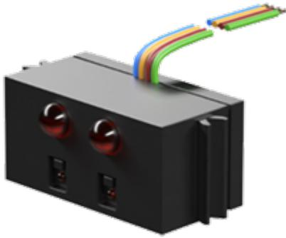
The infrared track sensor is a digital sensor used for detecting a black track on a white background, and works at a distance of 5 - 30 mm between the sensor and the background.
