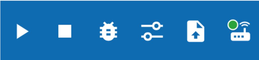
The header contains (from left to right) the operating elements for starting the program, stopping the program, starting the debugger, accessing the interface test, uploading the current program, and connecting to the Controller.
