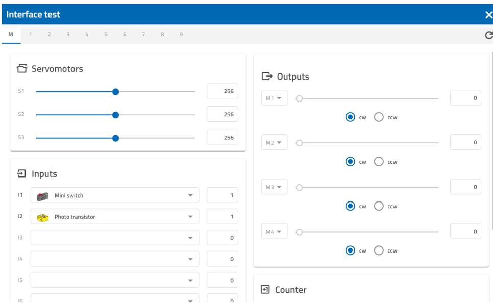
You can view all connected devices here. Under actuators, you can use the sliders to check whether they are working. The measured values are indicated for the sensors (there is a 1 by the button, for instance, because it is pressed). You can use the drop down menu (small triangle) to indicate what is connected.
